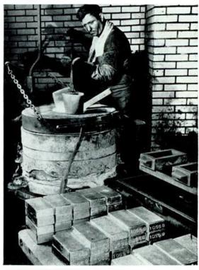
This is a foreign "mell." Gold from overseas arrives in bricks of varying sizes, must be melted down and made up into the standard bars you see opposite. This furnace is a big one. It melts 10,000 ounces of gold at one time. Its temperature must be  $2,000^{\circ}$  Fahrenheit. At a lower temperature gold will not pour properly, at a higher one too much will go off in smoke and fumes.
